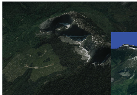
3D/DEM Production: 50cm DTM created from high resolution aerials
