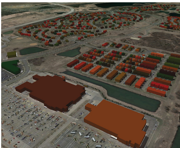
2.5D in Google Earth: Buildings extracted from aerial photography and 3D rendering accomplished with state-supplied LiDAR data (Scott County, MN)
